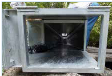
An underwater video recording box specially designed for the fishway.
